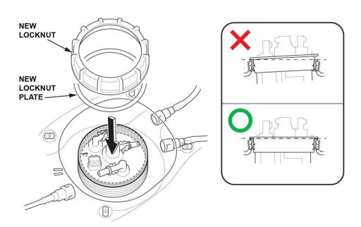
15.2. Tighten the fuel tank unit locknut to the specified torque using the fuel sender wrench.
