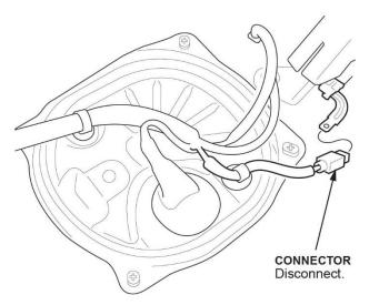
8.2. Remove the access panel from the floor.
