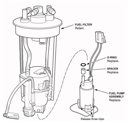
13. Assemble the fuel tank unit.
