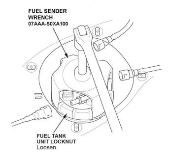
11. Remove the fuel tank unit locknut, then remove the fuel tank unit.
