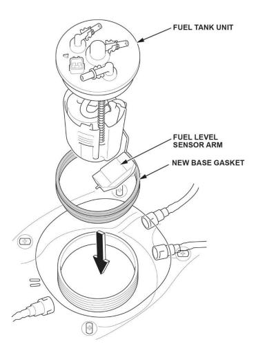
14.2. Line up the marks on the fuel tank and fuel tank unit as shown, then partially install the fuel tank unit.
