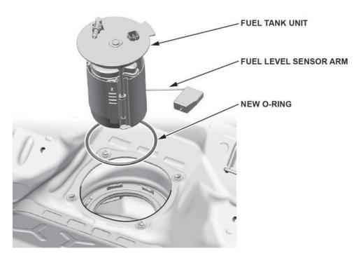
10.2. Line up the tab of the fuel tank unit as shown, and temporarily insert the new fuel tank unit cam lock ring.
