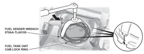
7.2. Turn the fuel tank unit cam lock ring counterclockwise.
