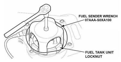
7. Remove the fuel tank unit locknut, and remove the fuel tank unit.
