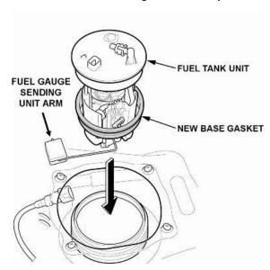
10.2. Line up the marks on the fuel tank and fuel tank unit, then insert the fuel tank unit into the fuel tank.
