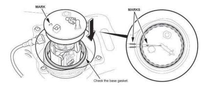
11. Tighten the fuel tank unit locknut.
