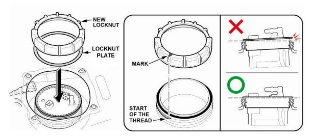
11.2. Tighten the fuel tank unit locknut to the specified torque using the fuel sender wrench.
