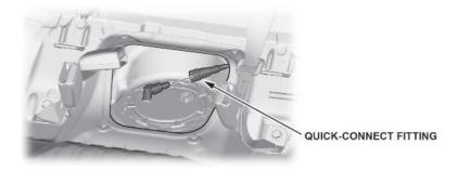
15. Connect the fuel tank unit connector.
