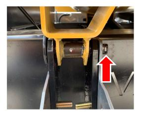
**3.** Push the headed pins out to be flush with the inner side of the tank hinges. Be careful not to push the pin through the hinge.
