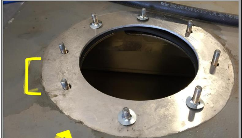
13. Use retaining washers purchased locally (NAPA 66525380) to HOLD the lower seal assembly in position
