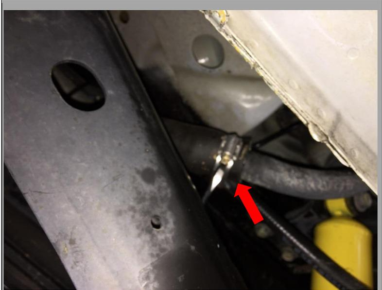
5. Locate the vapor canister located to the left of the fuel tank. CAREFULLY remove the UPPER vent line connector making sure not to damage either the connector or vapor canister.
