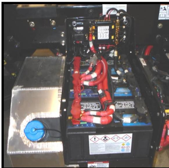
5. Verify with a voltmeter there is no voltage across the jumper studs.
