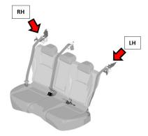
**IMPORTANT**: The use of **HAND TOOLS ONLY is strongly recommended** when performing these repairs. The use of air tools for bolt removal or installation may result in thread or weld nut damage. Weld nut damage may result in costly body panel replacement and would not be a matter for warranty. Work **CAREFULLY** using **hand tools only** along with a properly calibrated torque wrench to ensure all bolts are tightened and torqued to proper specification as part of this repair procedure.
