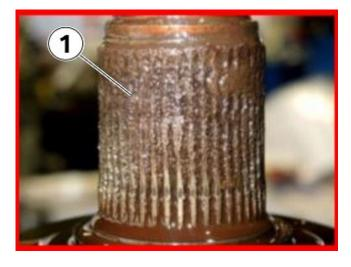
**NOTE:** The transfer case needs to be replaced if <u>either</u> the flange or the output shaft are worn.
