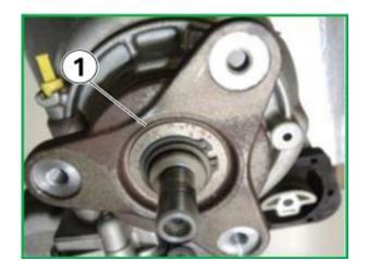
Typical output flanges without friction rust build up (1).
