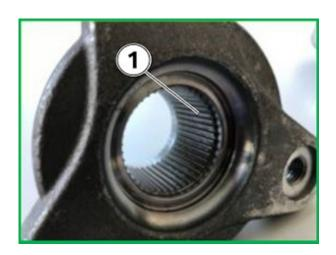
Typical flange and output shaft **without** any friction rust damage (1). Reinstall the flange (with new radial oil seal, O-ring and retaining ring) and reassemble the vehicle with new flex disc.
