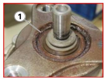
If rust build up cannot be determined by visual inspection, the flange will need to be removed for further diagnosis.
