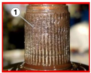
Flange and output shaft **with** friction rust damage (1). The transfer case will need to be replaced (with new flex disc).
