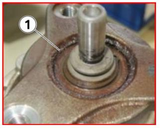
Output flanges with friction rust (1). Flanges with excessive friction rust will require transfer case replacement.
