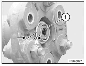
**IMPORTANT NOTE:** The centering bushing (1) needs to be pressed in to properly fit with the new (GS 105) flex disc.
