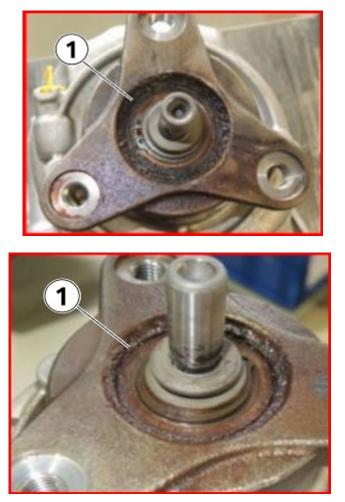
Output flanges with friction rust (1). Flanges with excessive friction rust will require transfer case replacement.
