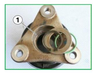
No further repair is necessary if there is no friction rust around the splines of the output flange.
