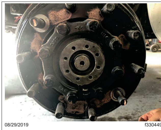
Fig. 3, Hub Cover Removed
