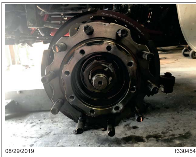
Fig. 9, Brake Drum Removed
