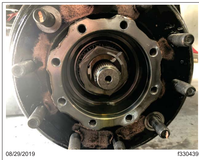
Fig. 8, Drive Flange from the Hub Removed
