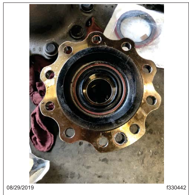
Fig. 22, Spindle Seal Installed
