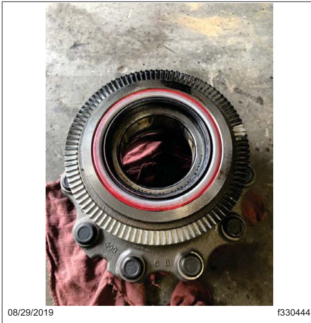
Fig. 25, Hub Seal Installed
