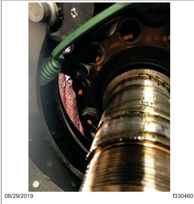
Fig. 15, Removal of ABS Sensor
