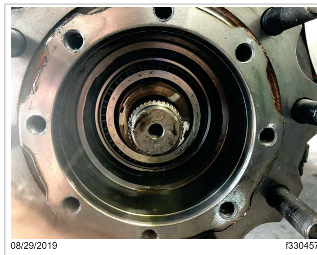
Fig. 12, Inner Spindle Nut Removed
