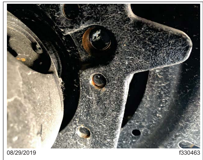
Fig. 18, ABS Sensor Removed
