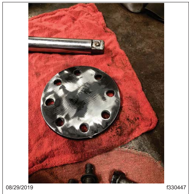
Fig. 28, Hub Cover Cleaned
