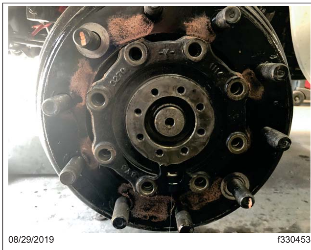
Fig. 7, Flange Bolts that connect the Drive Flange to the Wheel Hub Removed
