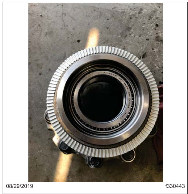
Fig. 24, New Inner Wheel Bearing Lubricated
