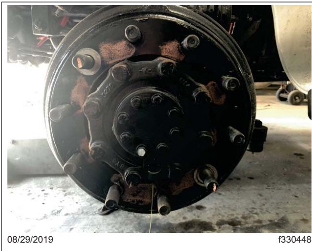
Fig. 1, Oil Fill/Drain Plug Removed
