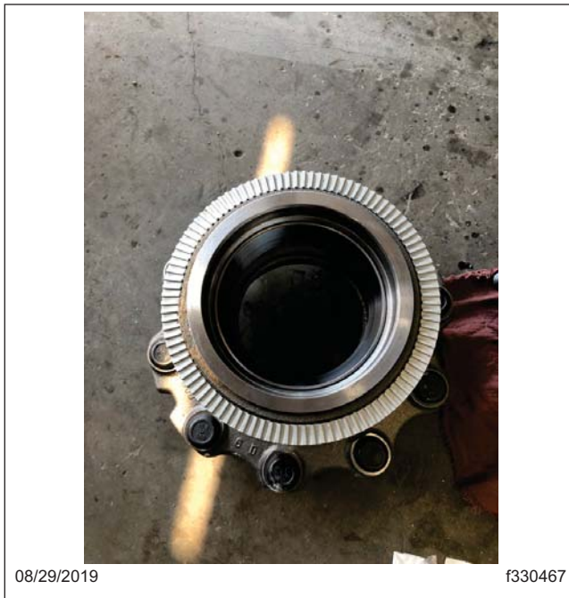
Fig. 23, Lubricating the New Inner Wheel Bearing
