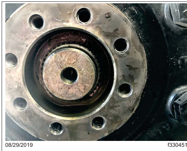
Fig. 5, Snap Ring Removed from Axle Shaft
