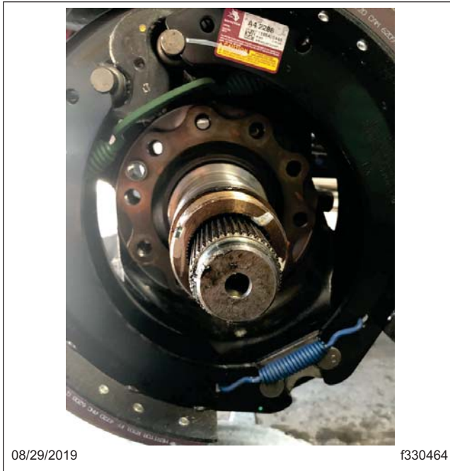
Fig. 19, Mounting Flange Bolt Removed
