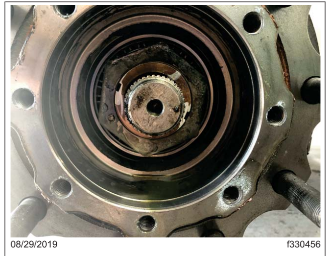
Fig. 11, Lock Ring Removed
