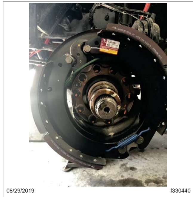
Fig. 14, Hub and Inner Bearing Removed
