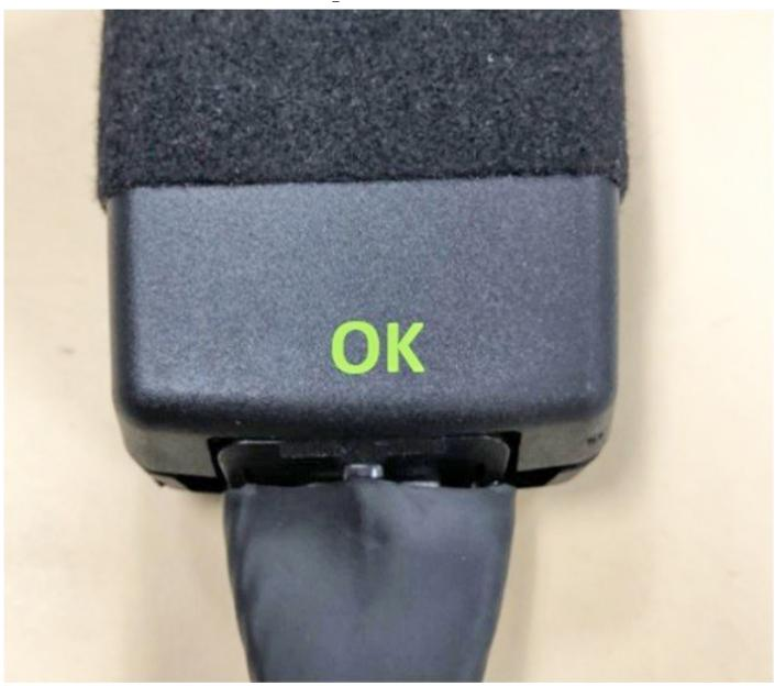
If there is a visual gap between the hall switch assembly and the buckle, replace the part.
