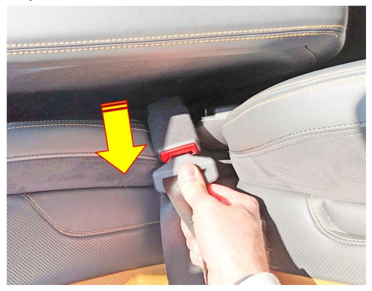
Inspect the <u>bottom</u> of the buckle. If needed for better access, bend the buckle forward. The hall switch connection is at the arrow.
