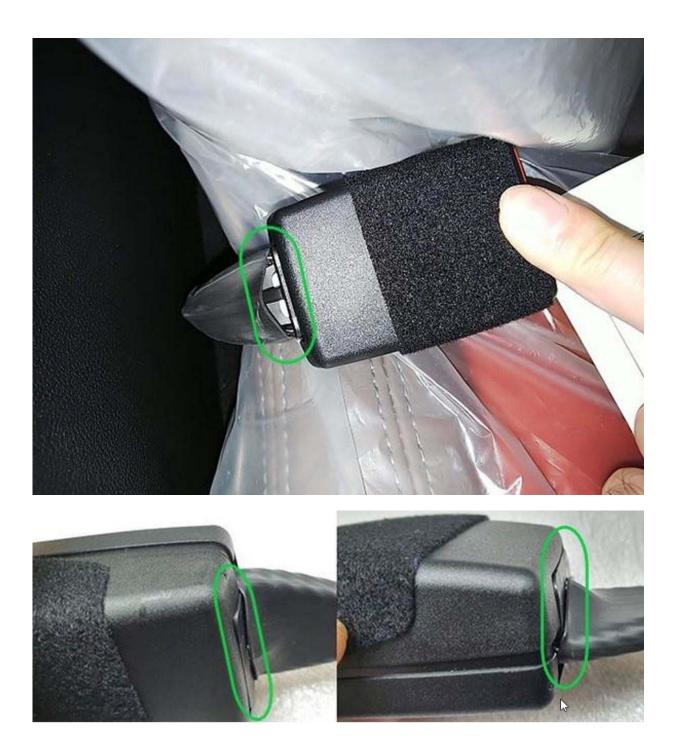
If there is a 3 mm or larger visual gap between the hall switch assembly and the buckle, replace the part.
