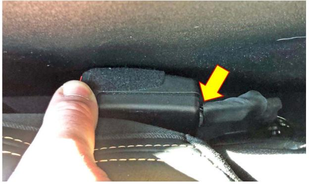
Verify visually if the hall switch remains in the correct position. Movement UP TO 3 mm is acceptable.
