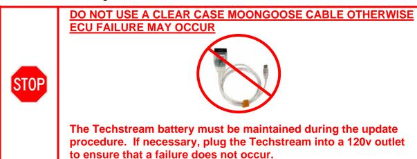
Note: If the Techstream communication with the vehicle fails during the re-flash procedure, the Engine ECU will be damaged and must be replaced.
