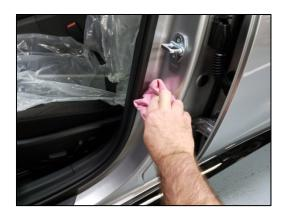
2. Apply the new Tire Specification Label directly on top of incorrect label.
