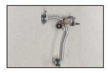
Using a long nose plier, carefully pull to remove the damper (F) inserted inside the delivery pipe as shown and <u>set aside</u> <u>as it will be re-used</u>.
