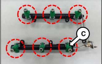
Note: Injector caps (H) should only be replaced if needed/damaged. Lubricate o-rings when installing.
