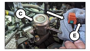
5. Remove/detach the three (3) upper fuel line (E) retaining brackets (2.4L shown).
