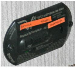
Unit will not have a separate C/O detector (pictured on 1<sup>st</sup> page) if it has this style LP-C/O detector (pictured above) in the unit. Units with this style LP-C/O detector cannot have the C/O and smoke detector switched and will require that an additional smoke detector be installed in the main body of the unit, if the smoke detector is located in the bedroom.
