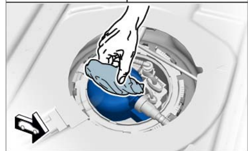
Cleaning top of filter flange of fuel pump
