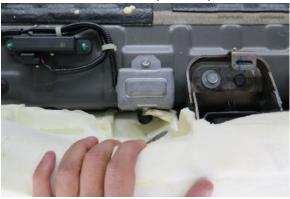
2. Loosen (halfway) the  ${\bf A}$  bolt, then remove the  ${\bf B}$  bolt.
