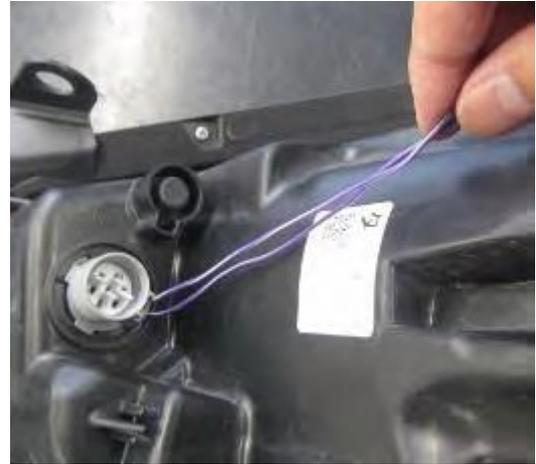
5. Unlock and make a gap between housing and connector.
