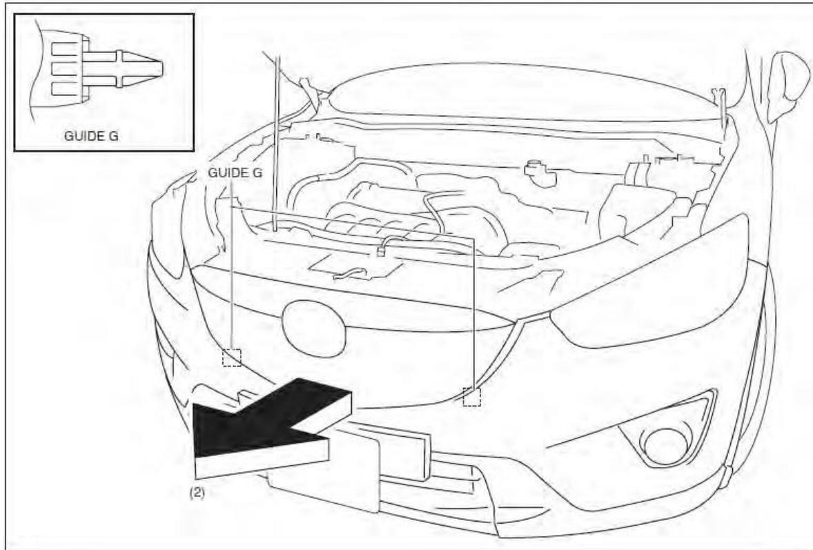
13. Disconnect the front fog light connector. (with front fog lights)
