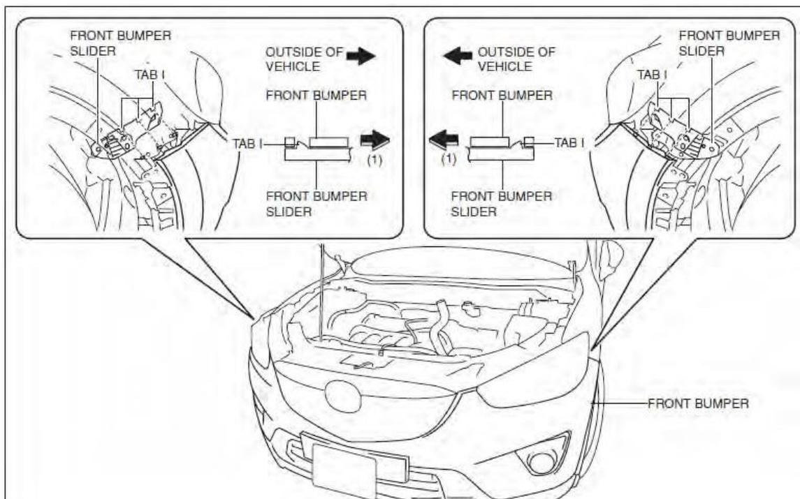
11. Remove the front bumper from the front bumper slider.
