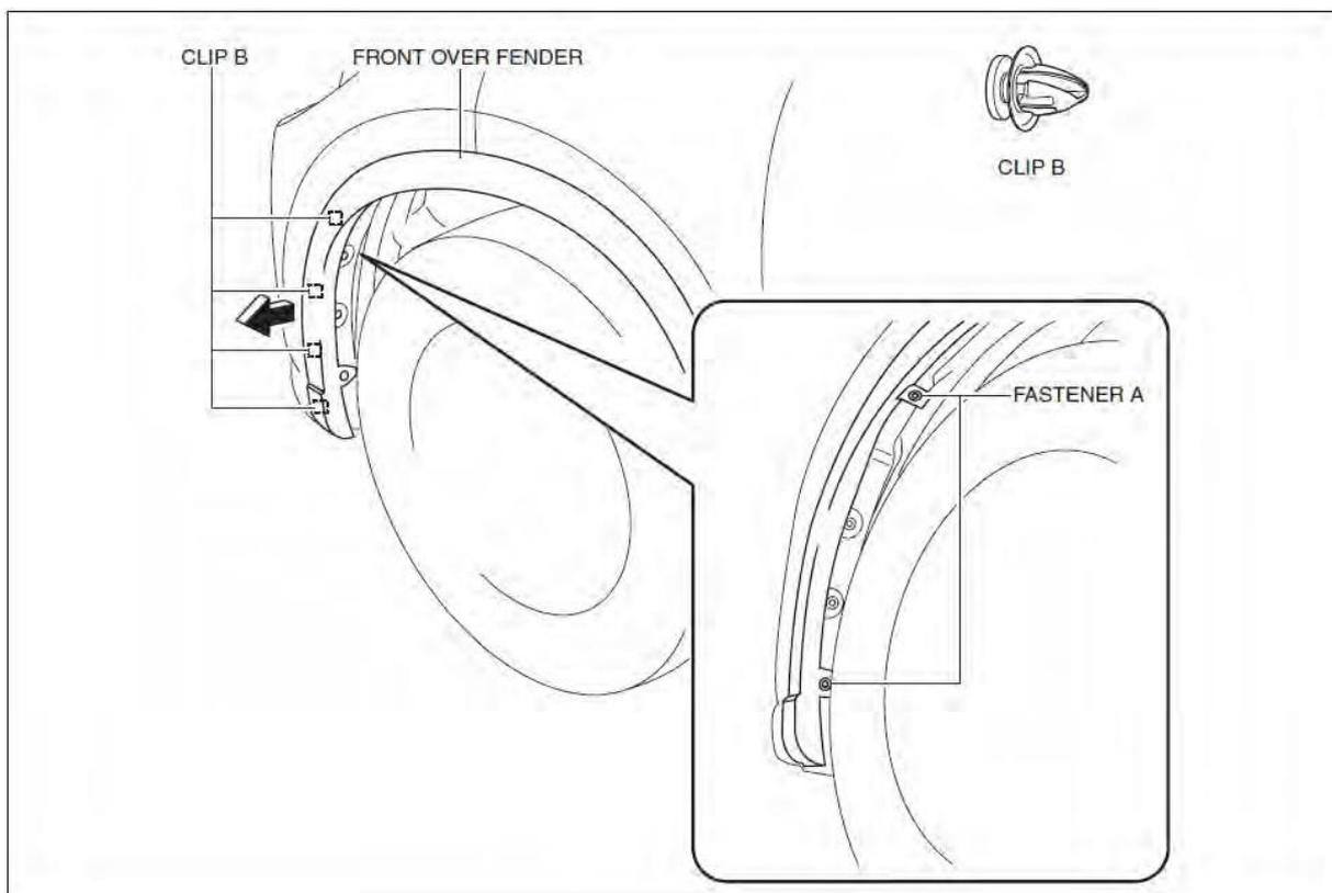
3. Pull the front over fender in the direction of the arrow shown in the figure, set the front over fender out of the way while detaching clips B.
