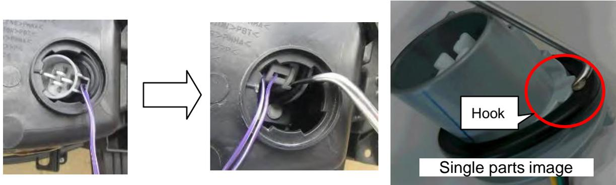
**Note: Connector A will not drop down far enough to turn 90 degrees. This O ring has limited room and visibility. Watch Video A**
