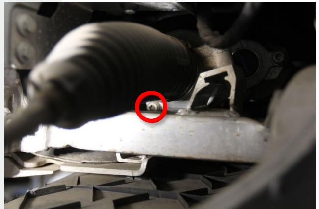
Figure 2 – Steering rack housing bolt 4
