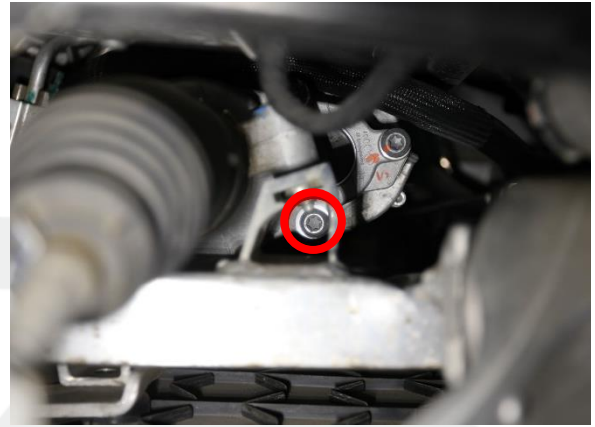
Figure 9 – Steering rack housing bolt 3
