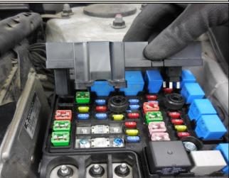
7. Install and tighten the fuse bolts (F).
