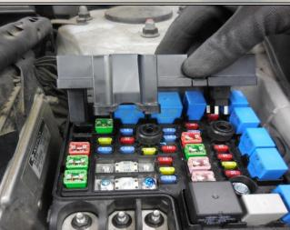
7. Install and tighten the fuse bolts (F). **Tightening Torque:** 3.9~4.9 Nm (0.4~0.5 kgf.m, 2.9~3.6 lb-ft)
