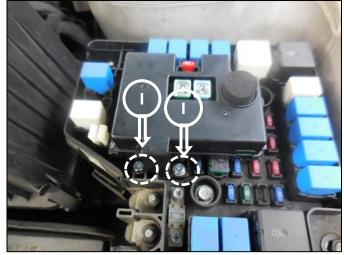
8. Remove the body ground bolt and reinstall it with the extension wire terminal (J) attached.
