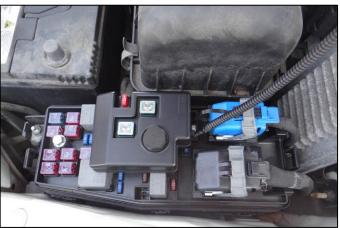
6. Route the extension wire (F) around the rear of the junction box to the battery in the gap (G) between the air cleaner housing and the junction box.
