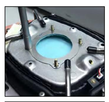
Press spacer on flush with airbag frame using a socket, for example.
