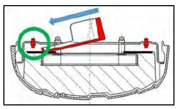
• Slide the rivet collector in at a slight angle and without resistance into the expanded gap.
