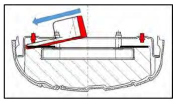
Continue to slide the rivet collector in at a slight angle and without resistance into the expanded gap, past the remaining portion of the pop rivet, until the rivet collector stops.
