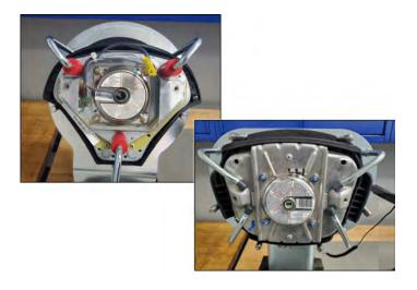
Inspect driver airbag inflator and replace if necessary.
