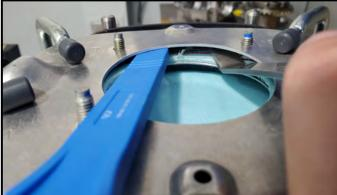
• Carefully pry open a gap so the -T10119- <A> can be inserted into the gap.
