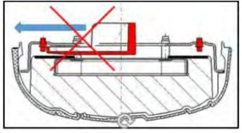
• Do not press the rivet collector against a rivet which has been drilled off.
