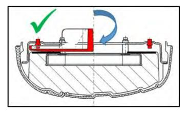
• Carefully rotate the rivet collector into the horizontal position.
