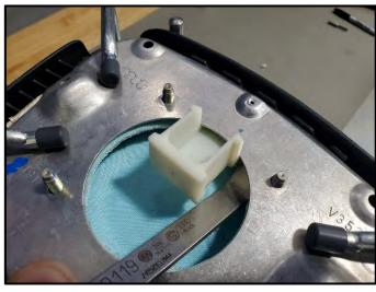
• Final installation positon of the rivet collector shown.
