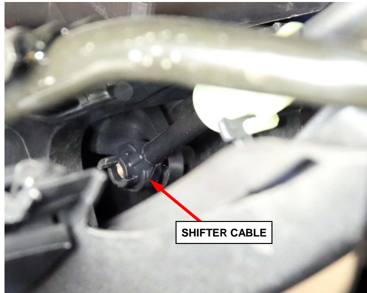
Figure 6 – Disconnect Shifter Cable from Shifter
