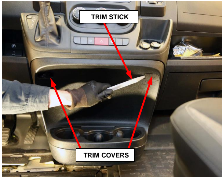
Figure 2 – Cup Holder Assembly Fasteners
