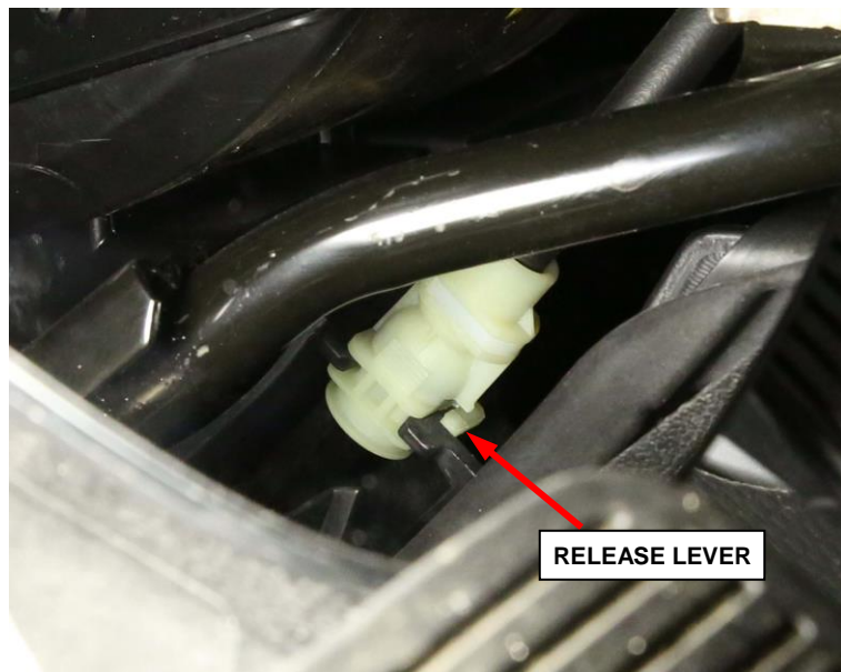
Figure 7 – Remove Shifter Cable Assembly from Shifter
