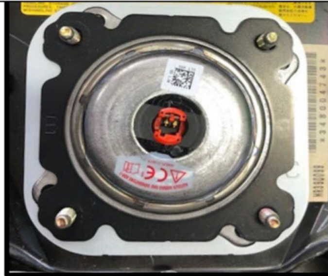
SAMPLE PHOTO OF CORRECT INFLATOR KIT ASSEMBLY
