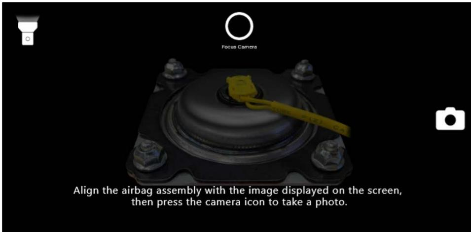
18. For the fourth photo, V-SMART will direct you to take a photo from angle 2. This view is looking from the top of the inflator at an angle with a clear view of the mating surfaces between silver plate A, black plate B, and the airbag assembly. Select **Continue** to proceed.
