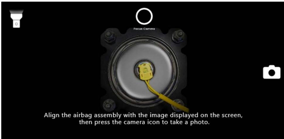
17. For the third photo, V-SMART will direct you to take a photo from angle 1. This view is looking from the bottom of the inflator at an angle, with a clear view of the mating surfaces between silver plate A, black plate B, and the airbag assembly. Select **Continue** to proceed.
