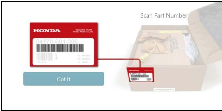
12. Scan the part number using the V-SMART camera.
