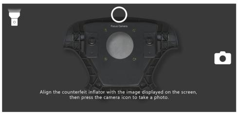
• If an unaffected M/D number is identified: V-SMART will direct you to take a photo of the airbag serial number label so it is clearly visible. Select **Continue** to move on to the photo for documentation.
