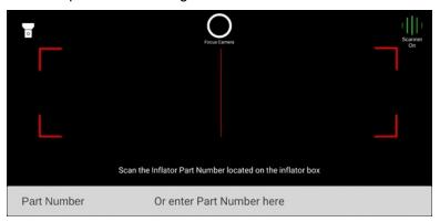
You can also enter the part number manually by selecting **Or enter Part Number here**. A keyboard will appear and you can enter the part number. Uppercase is not required to enter the part number correctly.
