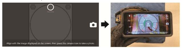
11. Confirm V-SMART has correctly identified the inflator label type. If it identified a green, blue, or red-and-white label, select **Continue**. Select **Back** to retake the photo.
