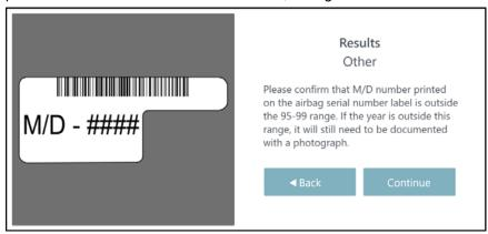
• If the label is missing or unreadable, the inflator is affected and must be replaced. Select **Continue**, or select **Back** to retake the photo.
