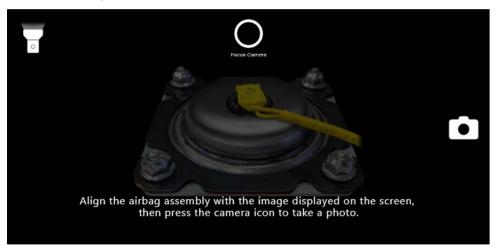
22. For the fourth photo, V-SMART will direct you to take a photo from angle 2. This view is looking from the top of the inflator at an angle with a clear view of the mating surfaces between silver plate A, black plate B, and the airbag assembly. Select **Continue** to proceed.
