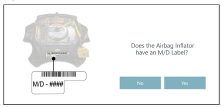
13. Hold the phone above the M/D label on the assembly and align the outline with the M/D label. Select the **Camera** icon to take a photo.
