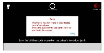
Select **Okay** to close the error. Then, select **Scanner Off** to reactivate the scanner, check the VIN, and try again. If you continue to see the errors above, do a VIN status inquiry to make sure the service bulletin applies to this vehicle.
