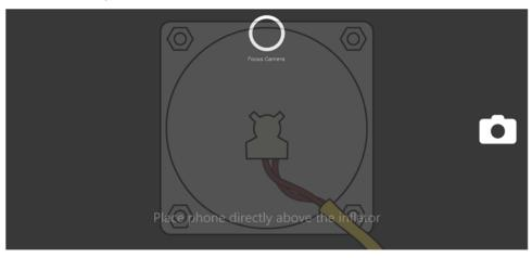
• If a counterfeit airbag assembly is identified: V-SMART will direct you to take a photo looking straight down at the airbag assembly so the inflator is clearly visible. Select **Continue** to move on to the photo for documentation.
