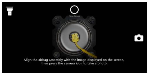
21. For the third photo, V-SMART will direct you to take a photo from angle 1. This view is looking from the bottom of the inflator at an angle, with a clear view of the mating surfaces between silver plate A, black plate B, and the airbag assembly. Select **Continue** to proceed.
