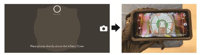
Confirm V-SMART has correctly identified the inflator cover type. If it has, select Continue. If not, select Back to retake the photo.
