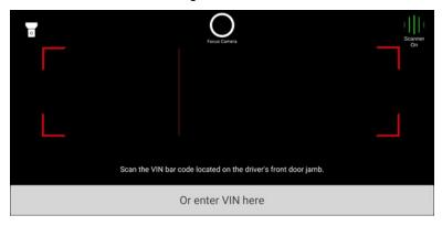
If the barcode is missing or damaged, you can also enter the VIN manually by selecting **Or enter VIN here**. A keyboard will appear, and you can type the VIN. Uppercase is not required when entering the VIN.
