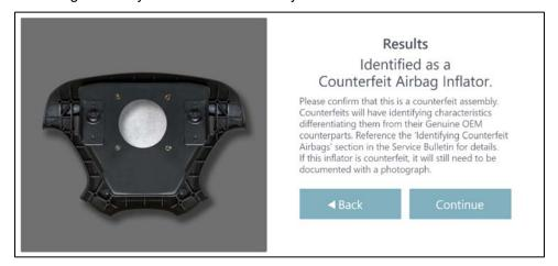
V-SMART will show an example of how to line up the airbag assembly to take the documentation photo. Select the **Camera** icon to take the photo.
