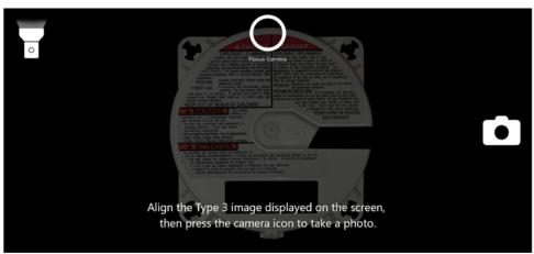
• If an unaffected inflator is identified: V-SMART will direct you to take a photo looking straight down at the airbag assembly with the cover clearly visible. Select **Continue** to move on to the photo for documentation.
