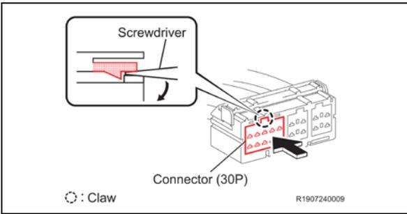
d) Using a screwdriver, disengage the claw and remove the connector (30P) from the connector holder.
