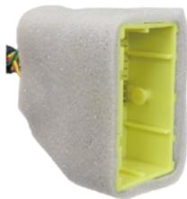
The sheet is **FLUSH** with the connector
