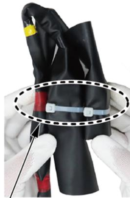
Align the vinyl tape with cable ties
