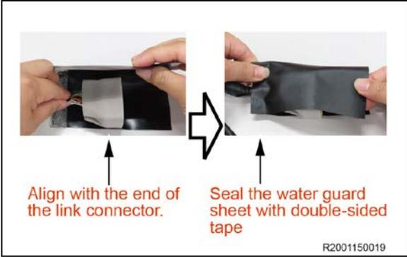
j) Remove the release paper of the double-sided tape.
