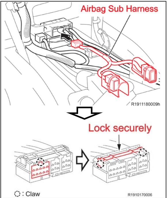
e) Connect the connector (30P) of airbag sub harness to the connector holder of the airbag sensor and lock the retainer securely.
