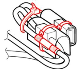
Be sure that place so that the part not protected by the sheets are on the underside of the vehicle.
