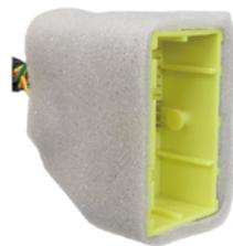
The sheet is **FLUSH** with the connector
