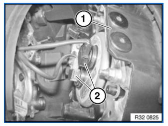
*Installation:* Connect plugs to connections of same colour on airbag unit.
