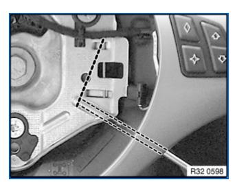
Insert Torx screwdriver (T25) at an angle into concealed opening on reverse side of steering wheel until a spring resistance is felt (approx. 1.5 cm).
