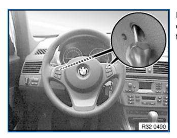
Insert Torx screwdriver (T30) horizontally into opening on reverse side of steering wheel up to stop (approx. 4.5 cm).
