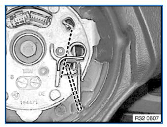
Insert Torx screwdriver (T20) roughly straight from below into opening on reverse side of steering wheel up to stop (approx. 5.5 cm).
