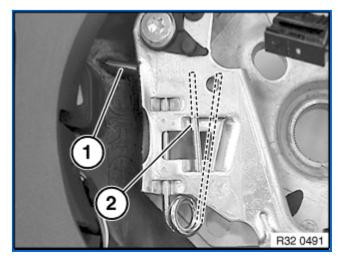
Increase pressure with Torx screwdriver T30 (1) on spring leg (2) until airbag unit is unlocked.
