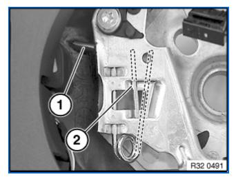
Increase pressure with Torx screwdriver T30 (1) on spring leg (2) until airbag unit is unlocked.
