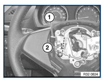
Insert Torx screwdriver T30 (1) horizontally into opening on reverse side of steering wheel until a spring resistance is felt (approx. 4 cm).
