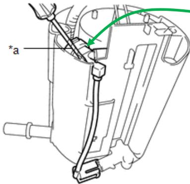
Repair Manual: Using a screwdriver (\*a) with its tip wrapped in protective tape, remove the jet pump from the No. 1 fuel sub-tank.
