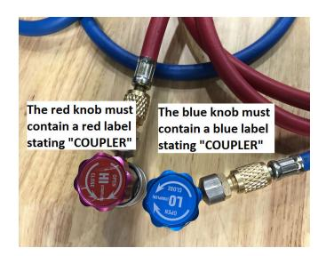
Once corrective labels have been applied, you may resume use of your AC Manifold Gauge Set. If your manifold gauge set already has labels in the correct positions you don't have to do anything and can discard the labels you received.
