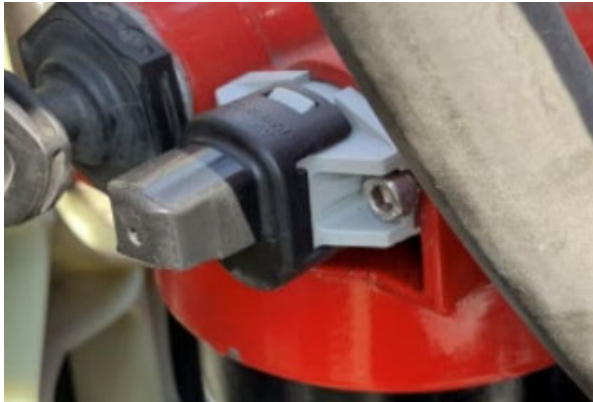
Figure 2: Fuel Heater Connector Cut
