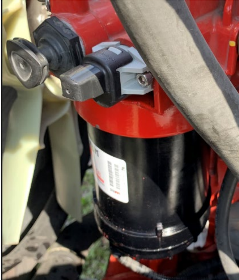
Figure 12: Fuel Heater shown after cutting complete
