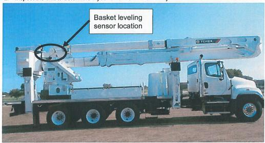
a. Remove cover by removing the two polytop screws to access the basket level sensor.
