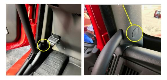
2. Remove fastener holding panel in place
