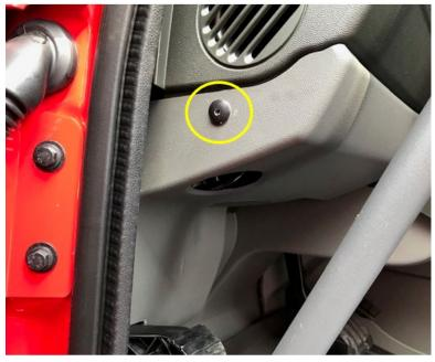
10. Install grab handle, torque fasteners to 18 +/- 3 foot pounds.
