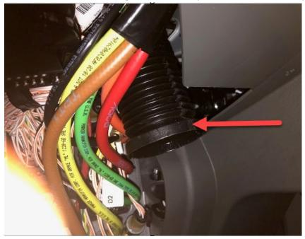
5. On each air hose at the pass through connection, one at a time, push in twice, and then pull out firmly.
