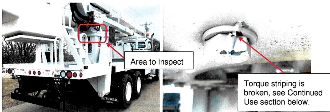
Figure 1. Area of unit to inspect rotation bearing bolts
