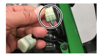
Connect KVCI device to vehicle's white, six pin FI ECU connector, using cable 57001-1843.
