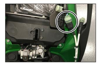
• Slide the **power switch** on the KVCI device to the **ON** position.
