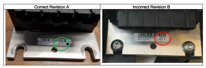
Please ensure the incorrect Rev B DC-DC converter is marked to avoid potential mix-up and contact the Zero Motorcycles Customer Service or Aftersales team to have a call tag generated to support the return shipment of the replaced converter to Zero Motorcycles.
