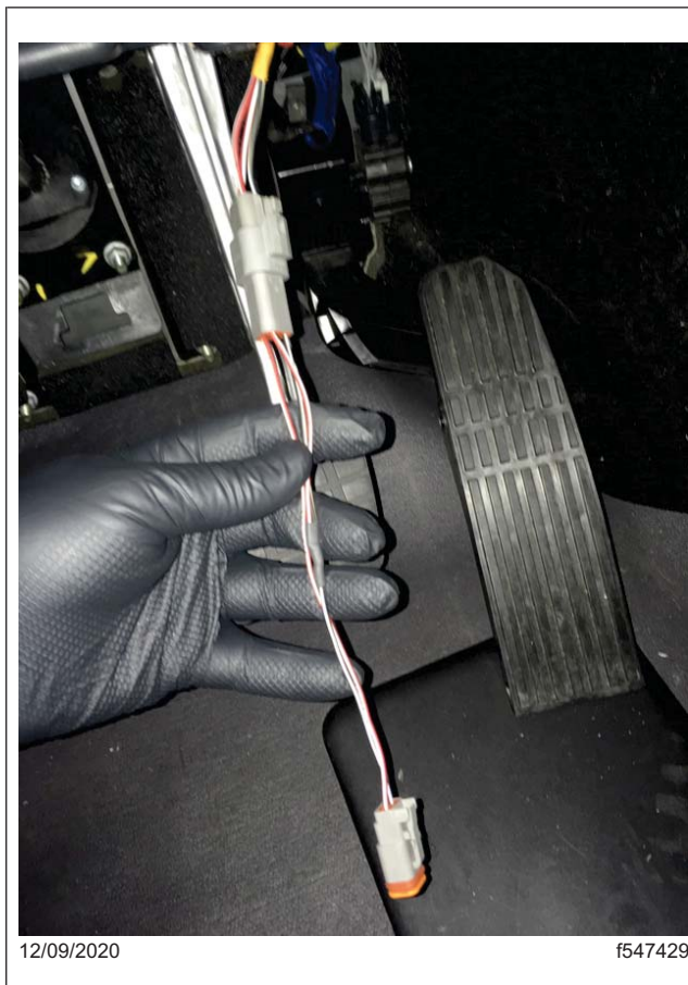
Fig. 4, Jumper Harness Connected to Cab Harness
