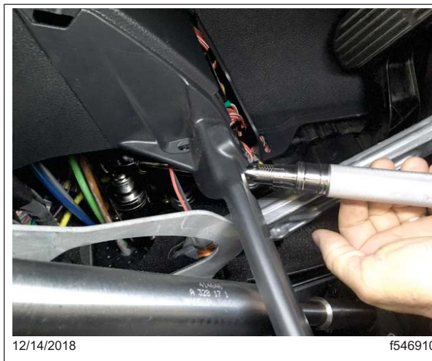
Fig. 2, Tightening the Brake Light Pressure Switch
