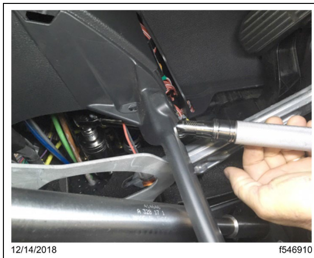
Fig. 2, Tightening the Brake Light Pressure Switch
