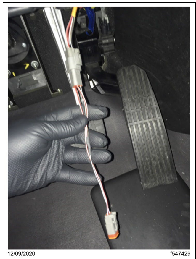
Fig. 4, Jumper Harness Connected to Cab Harness
