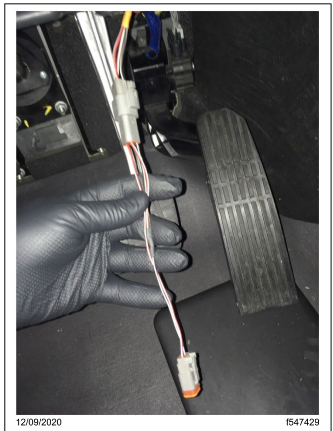
Fig. 11, Jumper Harness Connected to Cab Harness
