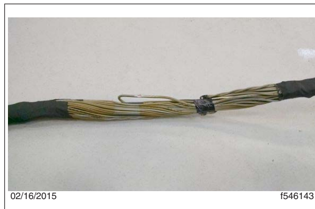
Fig. 7, Overlay Added to Damaged Area of the Harness
