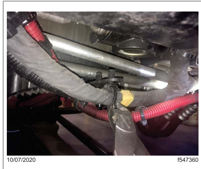
Fig. 2, Harness Tie Strap Removal
