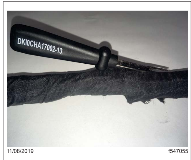
Fig. 5, Cutting the Fiber Wrap Using the Blunt End of the Seam Ripper
