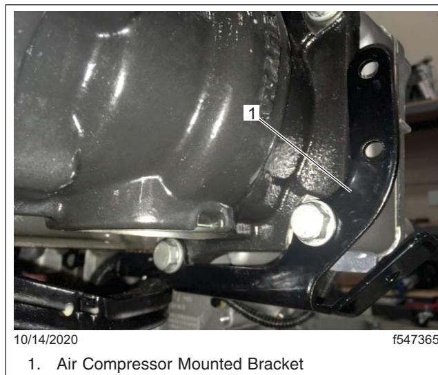
Fig. 15, New Air Compressor Mounted Bracket, Front View
