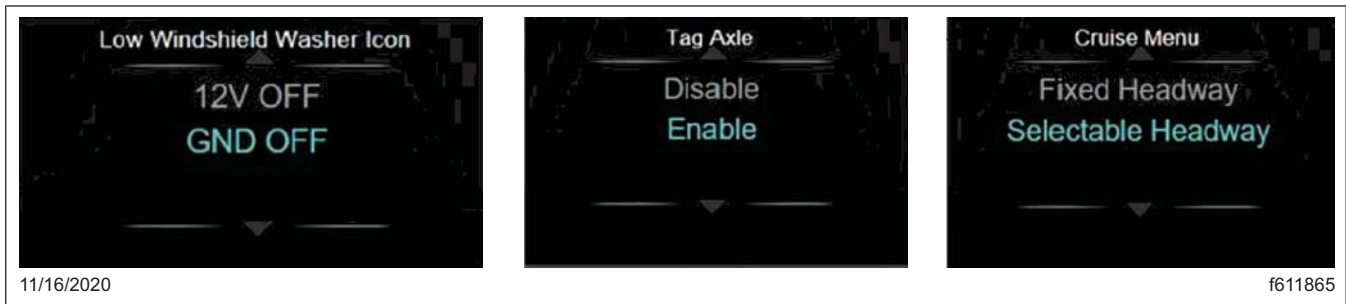
Fig. 15, HMI Configuration Menus (Group 2)
