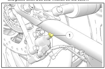
Loosen the rear foot control fastener so the foot control can be rotated.
