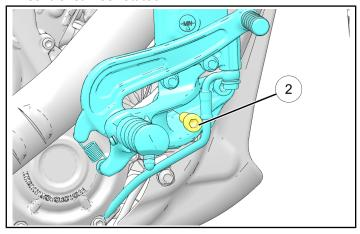
3. Rotate the foot control toward the front of the unit roughly twenty degrees to aid in removing any possible trapped air within the circuit.
