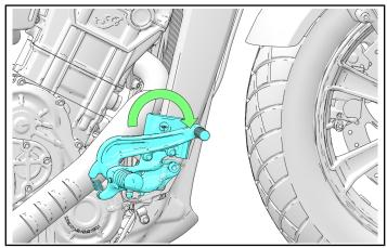
Clean and remove reservoir cap on the master cylinder.
