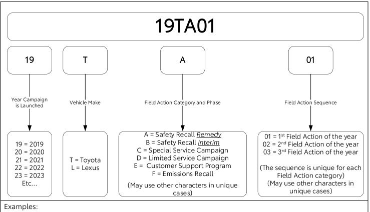
19TA01 = Launched in 2019, Toyota, Safety Recall Remedy Phase, 1<sup>st</sup> Safety Recall Launched in 2019 20TC02 = Launched in 2020, Special Service Campaign, 2<sup>nd</sup> Special Service Campaign Launched in 2020 21TE05 = Launched in 2021, Customer Support Program, 5<sup>th</sup> Customer Support Program Launched in 2021
